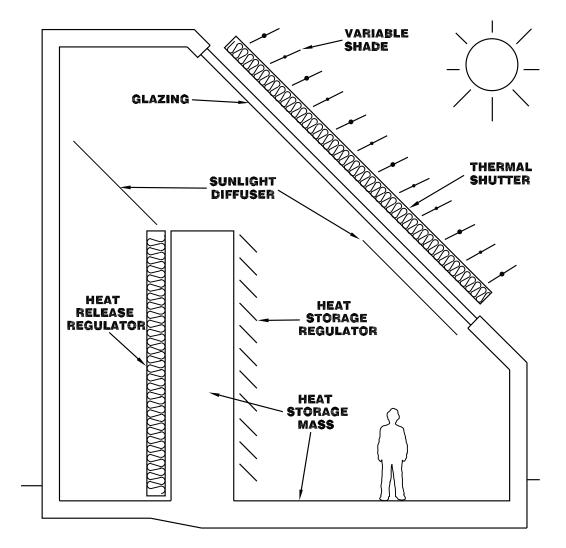
**Fig. 1 Complete passive solar heating system** This conceptual drawing symbolizes all the functions that any passive heating system should have. Bear in mind that any passive heating system is also a daylighting system, and it must perform well in both roles. In real installations, the clever designer will combine these functions wherever possible, and will exploit the inherent features of the building, such as heat storage mass.
