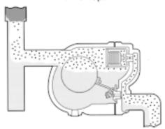
As air accumulates in the trap, the temperature drops below that of saturated steam. The balanced pressure thermostatic air vent opens and discharges air.
