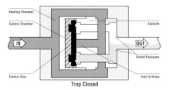
2. When steam reaches the disc, increased flow velocity across the face of the disc reduces pressure at this point, and the disc closes the orifice. Controlled bleeding of steam from the control chamber causes the trap to open. If condensate is present, it will be discharged. The trap recloses in the presence of steam and then continues to cycle at a controlled rate.
