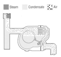
On start-up low system pressure forces air out through the thermostatic air vent. A high condensate load normally follows air venting and lifts the float which opens the main valve. The remaining air continues to discharge through the open vent.
