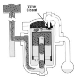
As the entering condensate starts to fill the bucket, the bucket begins to exert a pull on the lever. As the condensate continues to rise, more force is exerted until there is enough to open the valve against the differential pressure.
