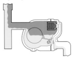
When steam reaches the trap, the thermostatic air vent closes in response to higher temperature. Condensate continues to flow through the main valve which is positioned by the float to discharge condensate at the same rate that it flows to the trap.
