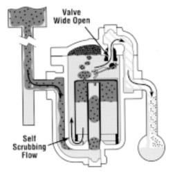
4. As the valve starts to open, the pressure force across the valve is reduced. The bucket then sinks rapidly and fully opens the valve. Accumulated air is discharged first, followed by condensate. The flow under the bottom of the bucket picks up dirt and sweeps it out of the trap. Discharge continues until more steam floats the bucket, and the cycle repeats.
