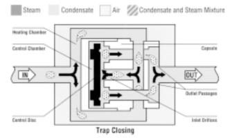
On start-up, condensate and air entering the trap pass through the heating chamber around the control chamber and through the inlet orifice. This flow lifts the disc off the inlet orifice, and the condensate flows through to the outlet passages.
