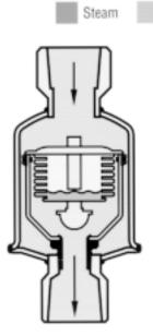
On start-up, condensate and air are pushed ahead of the steam directly through the trap. The thermostatic bellows element is fully contracted and the valve remains wide open until steam approaches the trap.
