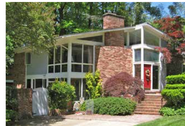
Figure 2-57. The window design of this house provides little privacy because the bottoms of the windows are at floor level. Without curtains or other privacy screens, the occupants have chosen to live in a public showroom.
