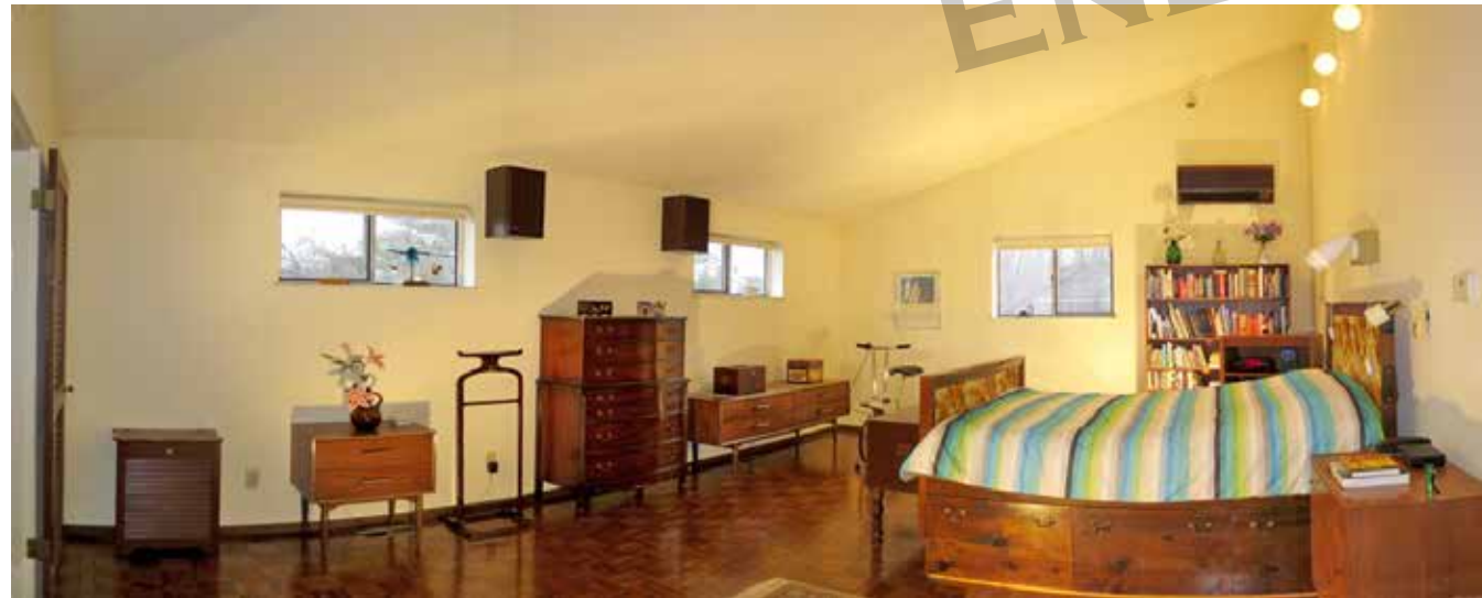
Figure 2-55. Tall window sills provide effective daylighting for this bedroom while maintaining privacy. The tall sills also allow furniture to be placed beneath the windows.
