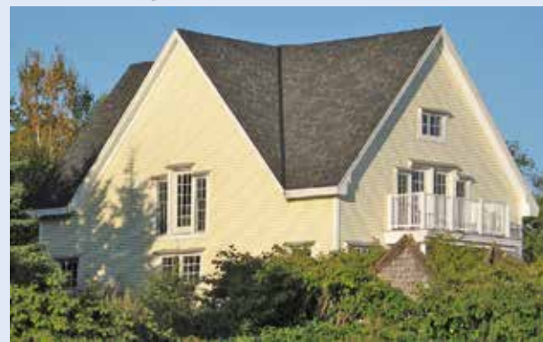
Figure 1-193. Cross gable roof. Gables of equal height meet in a cross pattern.
