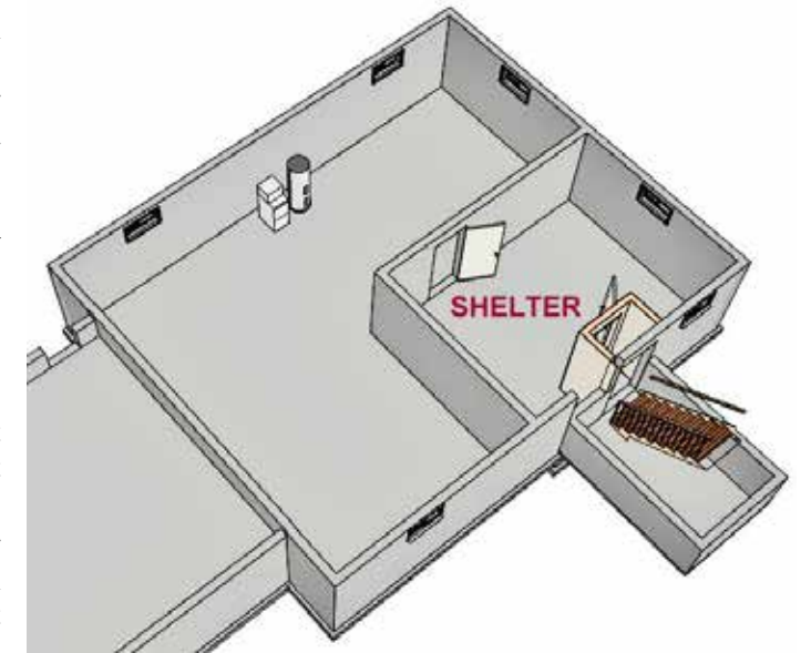
Figure 1-82. A basement emergency shelter that is completely surrounded by reinforced concrete walls. The walls provide strong support for the joists that form the ceiling. The shelter has direct access to the outside.
